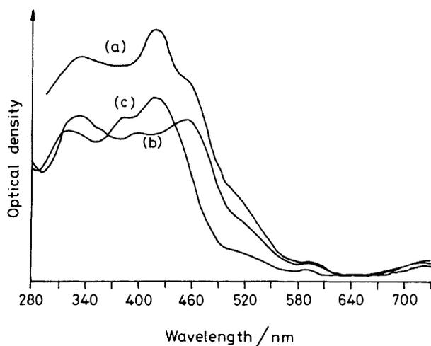
FIGURE. Electronic spectra in  $\text{CH}_2\text{Cl}_2$  of the intermediates generated from (a) FeTAPCl with PNPBA; (b) FeTAPCl with excess of CHP; (c) FeTTPCl with excess of CHP.
